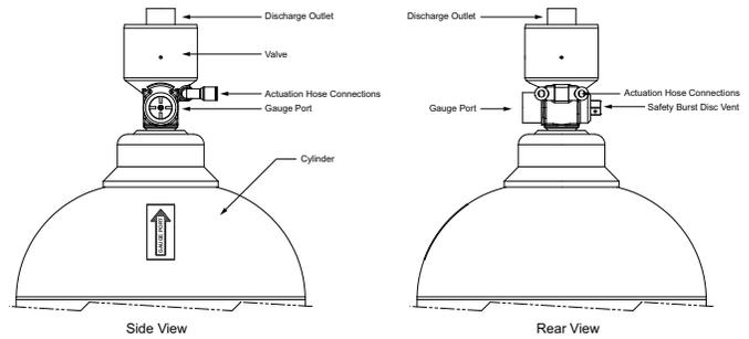
Figure 2. Valve General Arrangement,
